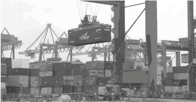
Fig. 15.6 Truck handling by a RMG crane
