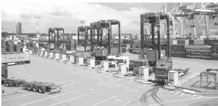
Fig. 15.5 Truck serving straddle carriers crane
