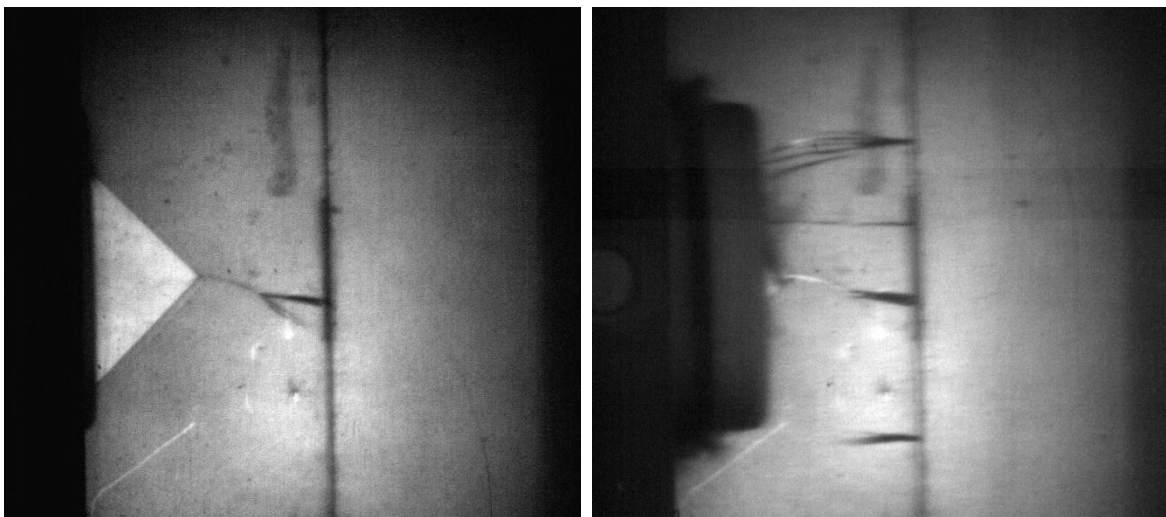
Figure 3. Crack propagation across an interface without adhesive (projectile: 217 g, 212 m/s, K.E.: 4880 J)
