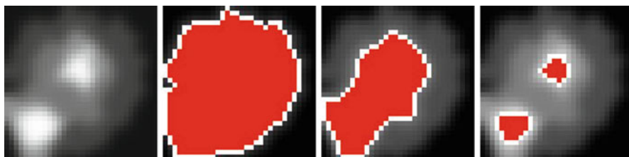
Fig. 13.1 “Area” feature for different threshold values in an 8-bit gray-level image. From left to right : original image; segmented area using a threshold of 55, 115, and 200. With increasing threshold value, the area is becoming smaller, and may even split into two disconnected regions
