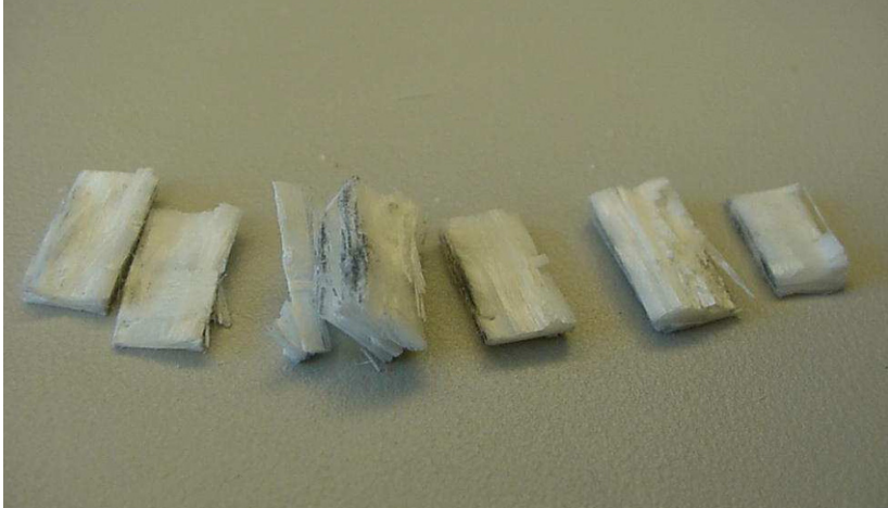
Figure 3.33 Composite specimen after mechanical loading along in-plane direction (Reproduced from Song et al. (2003) with permission)
