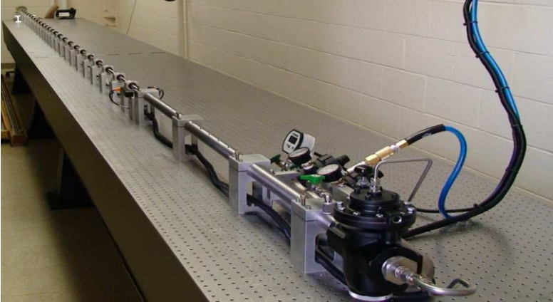
Figure 1.12 Photograph of the Kolsky compression bar (Reproduced from Song et al. (2009b) with permission)
