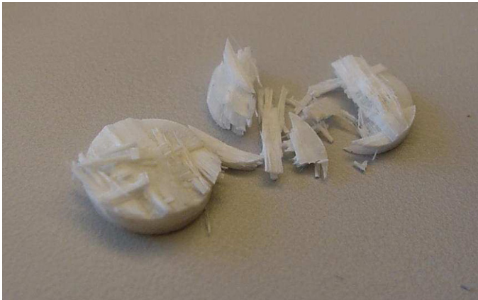
Figure 3.32 Composite specimen after mechanical loading along through-thickness direction (Reproduced from Song et al. (2003) with permission)
