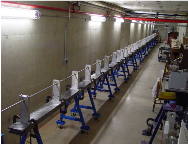
Figure 9.4 A photograph of a long Kolsky bar
