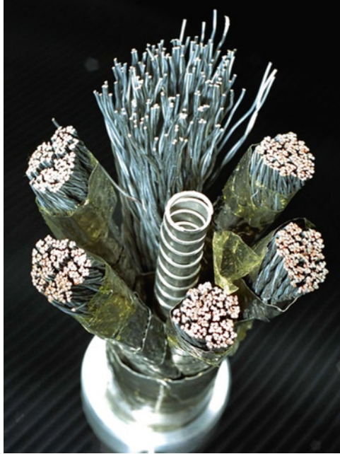
Fig. 9.21 Construction of a niobium-tin cable. One of the bundles has been exploded to show the strands [14]
