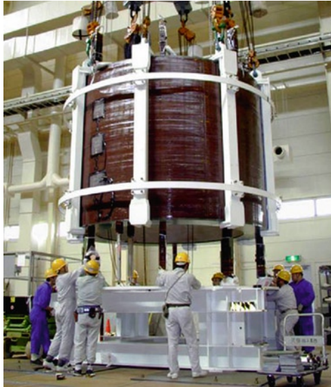
Fig. 9.23 A test section of the Central Solenoid for ITER [14]
