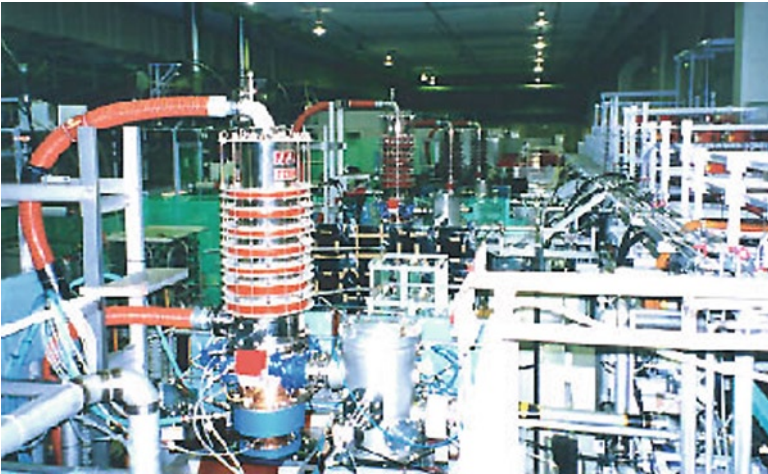
Fig. 9.24 The gyrotron room at JAERI [35]. A 1-MW gyrotron is shown at the left . It is 3 m (10 feet) high and covered with magnetic coils
