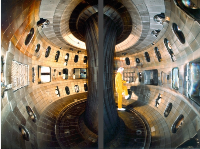
Fig. 8.7 Inside the vacuum chamber of DIII-D when it is opened up to air
