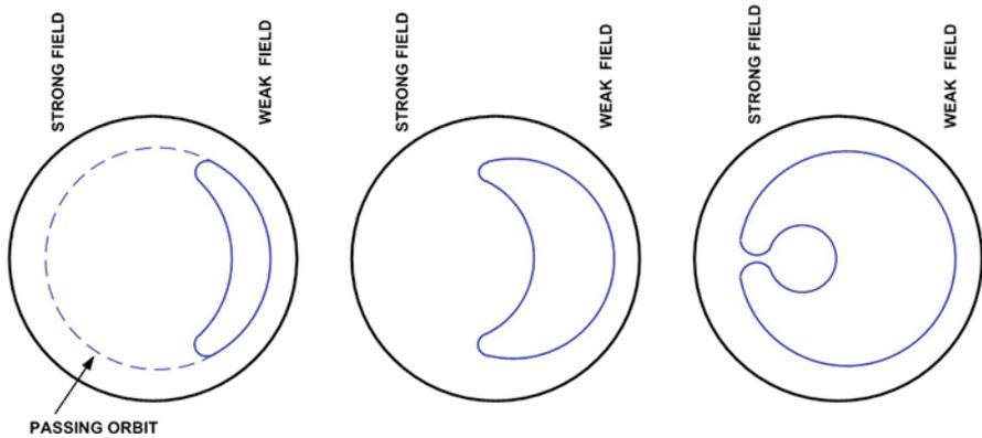
Fig. 6.6 Banana orbits of particles with increasing parallel velocities
