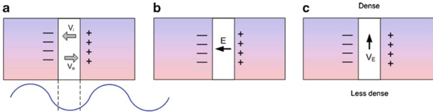
Fig. 6.15 The charges, fields, and velocities in the trough of a drift wave
