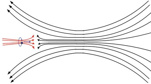
**Fig. 6.4** Reflection of an ion heading into a stronger magnetic field. The field generated by the ion's gyration is shown in *red*
