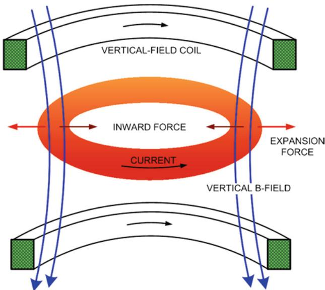
Fig. 6.19 Application of a vertical B-field to keep a ring of plasma from expanding
