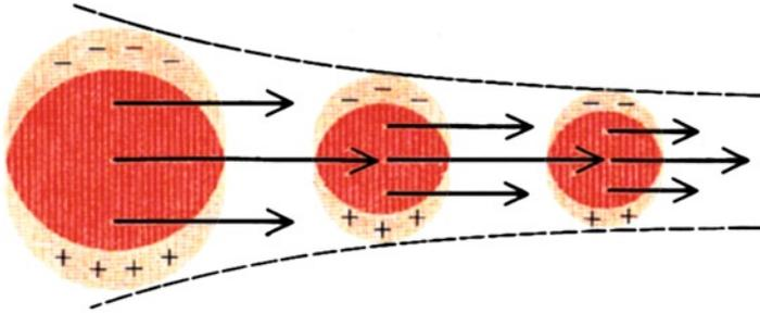
**Fig. 6.17** Anomalous transport of plasma in blobs (adopted from Chen [7]). These are not spheres but long tubes of plasma curving with the magnetic field lines
