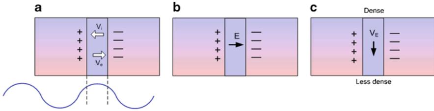
Fig. 6.14 The charges, fields, and velocities at the peak of a drift wave
