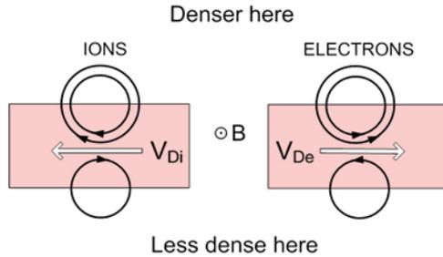
**Fig. 6.13** Definition of the diamagnetic drift. The electron orbits are actually much smaller than those of the ions
