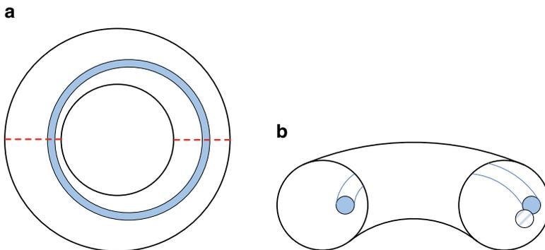
Fig. 6.3 A large kink distortion of the plasma in a torus: (a) top view and (b) cross-sectional view
