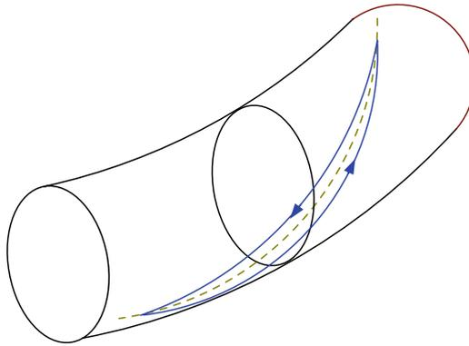
**Fig. 6.5** A banana orbit in a tokamak. In reality, this orbit drifts around the torus
