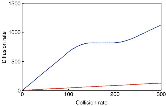
**Fig. 6.7** Neoclassical (*top curve*) and classical (*bottom curve*) diffusion rate for ions as a function of collision frequency<sup>3</sup>
