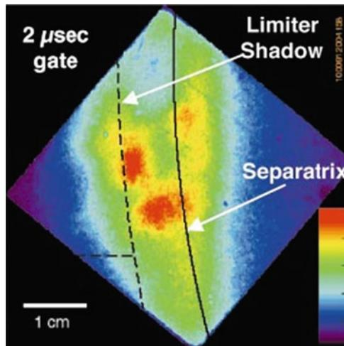
**Fig. 6.18** A picture of blobs leaving a tokamak, taken at a shutter speed of 2 millionths of a second. The outside of the torus is on the *left* [6]
