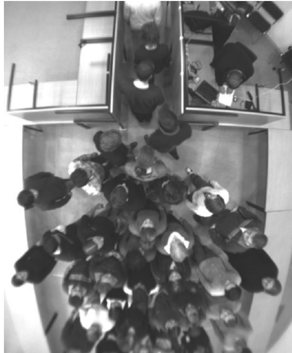
Evacuation Dynamics: Empirical Results, Modeling and Applications, Figure 1 Clogging near a bottleneck. The shape of the clog is discussed in more detail in Subsect. "Theoretical Results"
