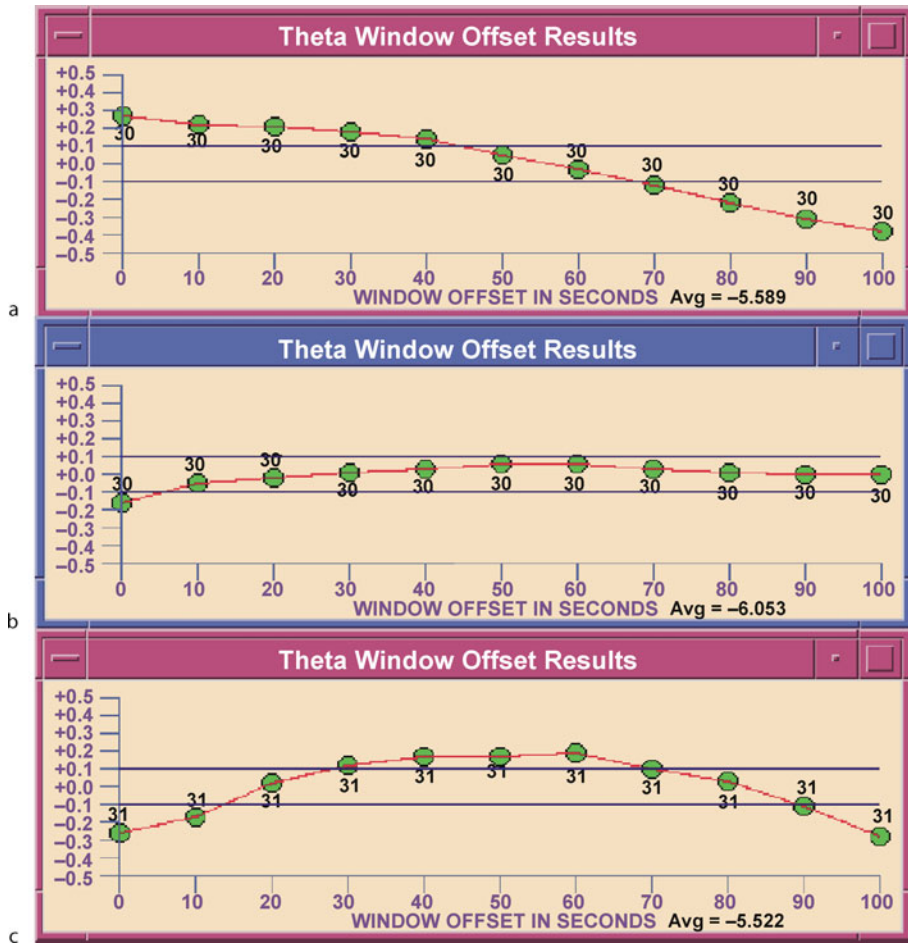
Earthquake Source Parameters, Rapid Estimates for Tsunami Warning, Figure 11 The variation of \Theta with offset for a “normal” earthquake, b a “slow earthquake” (Java, 2006), and c a complex earthquake (Peru, 2008) respectively. In these plots \Theta is de-meaned (the mean is found on the bottom right of the plot in black) and the number next to the dots indicates how many stations were used in computing that value. These plots are taken from PTWC’s operational software
