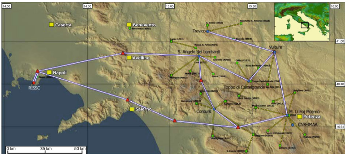
Earthquake Early Warning System in Southern Italy, Figure 3 Topology of the communication system of ISNet showing the extended-star configuration of the seismic network. Symbols explanation: green squares – seismic stations; blue squares – Local Control Centres (LCC); yellow lines – WLAN radio linkconnecting seismic stations and LCC; white segments – SDH carrier-class radio; red triangles – radio link repeaters; red circle – Network Control Centre RISS in Naples; yellow squares – main cities
