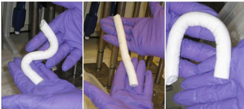
Figure 15.3. A di-isocyanate-reinforced wet gel with 35 mol% BTMSH -derived Si and 30 mol% Si from APTES is shown to be flexible and resilient before drying.
