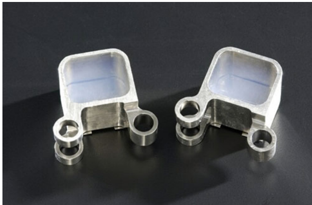
Figure 32.6. Proposed SCIM collection modules containing silica aerogel with a density of 20 mg/cc for hypervelocity particle capture.
