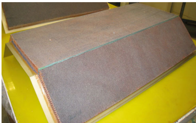
Figure 32.12. Heat exchanger panel for thermal stability of MSL MMRTG. MSL is scheduled to launch from the Kennedy Space Center in 2011 and land on Mars in 2012.
