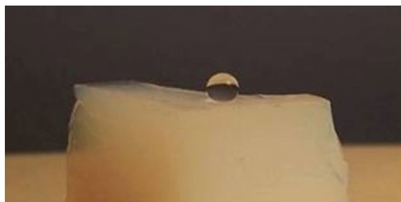
Figure 3.9. Image of a 2.5-mm diameter water drop on a hydrophobic silica aerogel monolith prepared using the co-precursor method with a mixture of TMOS and MTMS and RSCE drying.
