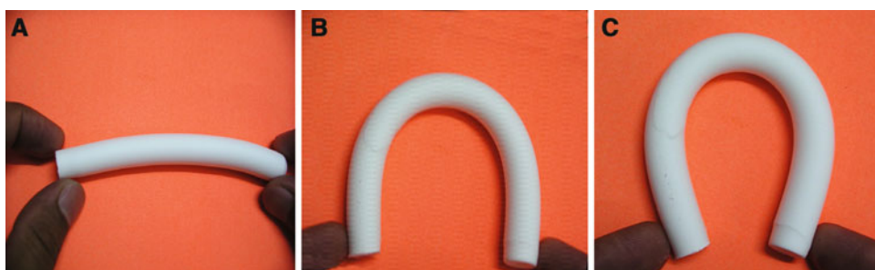
Figure 4.13. Photographs showing the maximum possible bending of the aerogels prepared at A. S = 6.45 , B. S = 12.96 , and C. S = 19.35 .
