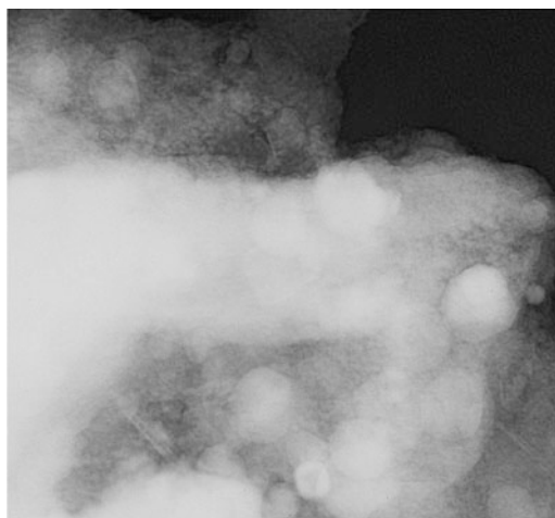
Figure 12.2. TEM micrographs of allophane aggregates. The width of the micrograph is 150 nm.
