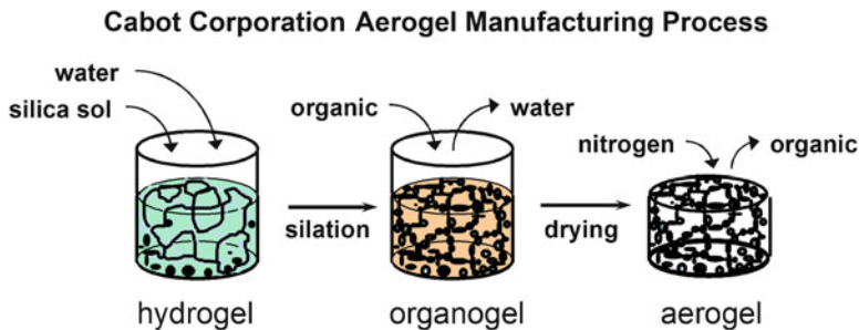
Figure 38.1. Schematic of Cabot's aerogel manufacturing process.
