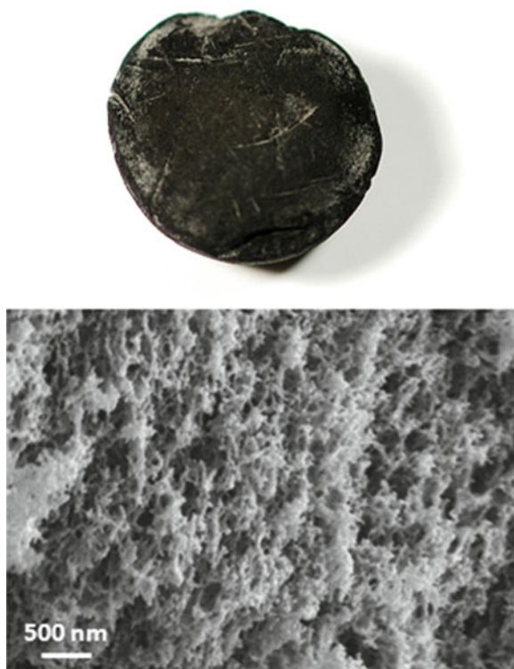
Figure 10.2. Carbon aerogels obtained from pyrolysis of cellulose aerogels. Top: optical photography (courtesy of T. Budtova, MINES ParisTech/CEMEF, Sophia Antipolis, France). Bottom: SEM (courtesy of M. Pinnow, Fraunhofer-IAP, Natural polymer division, Golm, Germany).
