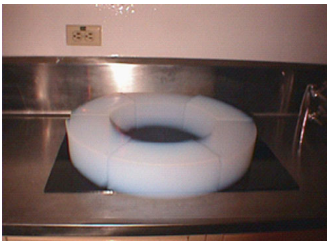
Figure 32.20. Prototype assembly of six rounded trapezoids. Outer diameter is approximately 50 cm.
