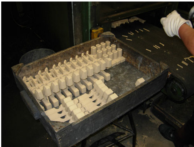
Figure 34.18. Core production in a foundry using m-silica aerogel as a nanoadditive (with permission of the company).
