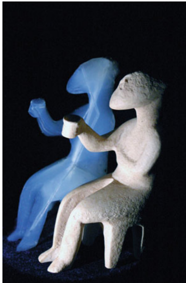
Figure 35.5. The cup-bearer . 15 \times 10 \times 7 cm. The silica aerogel sculpture weighs 20 g, but the marble sculpture weighs 350 g (photograph and copyright: MICHALOUS, 10/2006).
