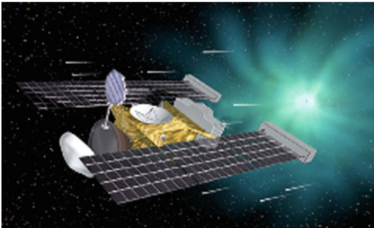
Figure 32.1. The aerogel is seen deployed extending above the spacecraft (left of center) for particle capture in this artist's image of the Stardust spacecraft.
