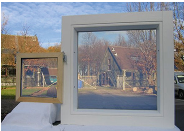
Figure 2.6. Large monolithic silica aerogel monoliths integrated in demonstration glazing ( left side ) and window ( right side ) prototypes [60]. Courtesy of K.I. Jensen and J.M. Schultz, DTU, Lyngby, Copenhagen.
