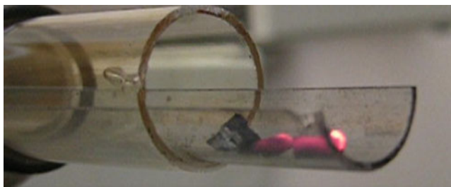
Figure 25.7. Photograph of the pyrophoric response of a nanostructured carbon/iron metal composite immediately after exposure to ambient atmosphere at ambient temperature. This composite has been measured to reach temperatures of ~650°C.
