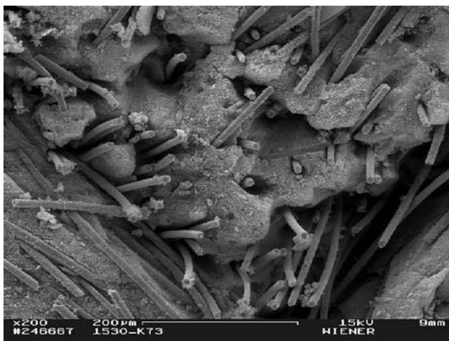
Figure 23.18. SEM image of a carbon-fiber felt with carbon-aerogel incorporated [45].
