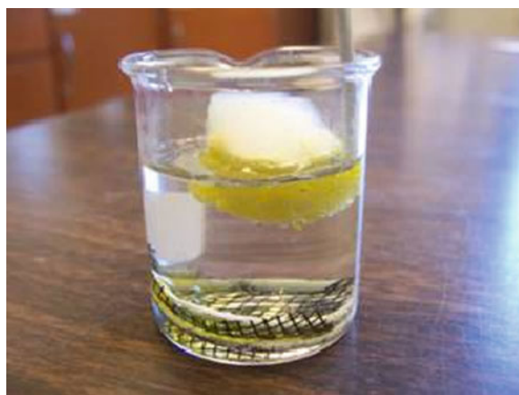
Figure 3.11. Demonstration of the oleophilic and hydrophobic nature of TMOS/MTMS aerogels. The aerogel monolith was placed in a beaker containing oil and water. Note that the aerogel has adsorbed the yellow oil, and is floating at the top of the water. The top part of the silica aerogel retains its optical properties, indicating that this aerogel had capacity to absorb additional oil. No oil layer is visible on the water surface.
