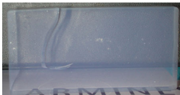
Figure 2.7. Typical depressurization crack (perpendicular to the largest surface) experimented by the silica gel during supercritical drying (illustrated here on a 1 cm thick wet silica tile having a liquid permeability between 5 and 10 nm 2 , dried with supercritical CO 2 at 313 K and 90 bar, and submitted to an autoclave depressurization of 0.15 bar min -1 ). Courtesy of Rigacci A.
