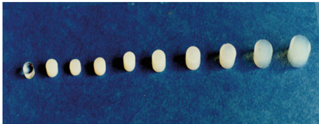
Figure 29.2. Set of partially sintered aerogels: from aerogel (relative density is 0.15, for the sample on the right) to fully sintered aerogel (transparent silica glass on the left, relative density is 1).
