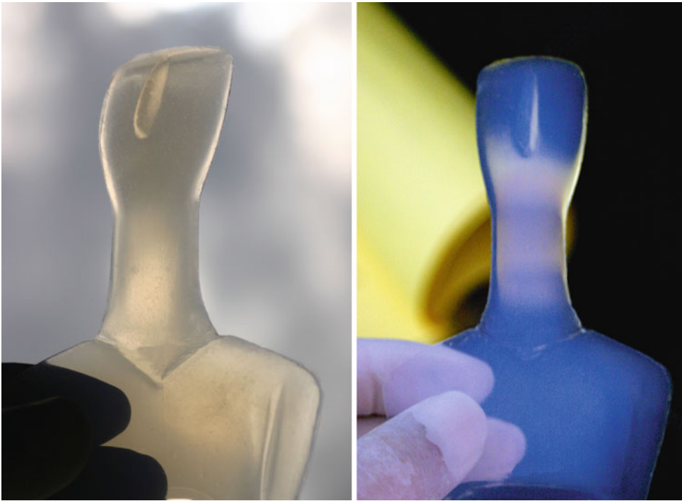
Figure 35.3. Leto , silica aerogel, 25 \times 15 \times 4 cm. In every aer( )sculpture , the orange golden hue is due to Mie scattering phenomenon and the blue one is due to the Raylight scattering phenomenon (photograph and copyright: MICHALOUS, 10/2006).
