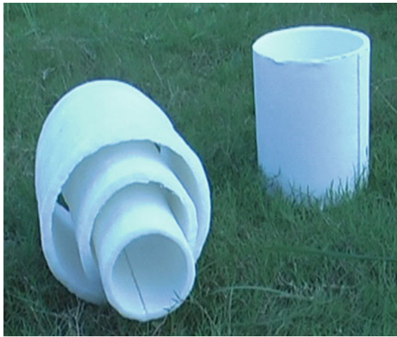
Figure 40.7. Thermal insulation cylinders.
