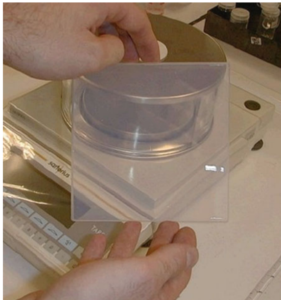
Figure 2.5. Monolithic silica aerogels obtained after supercritical CO 2 extraction. Courtesy of Rigacci A.
