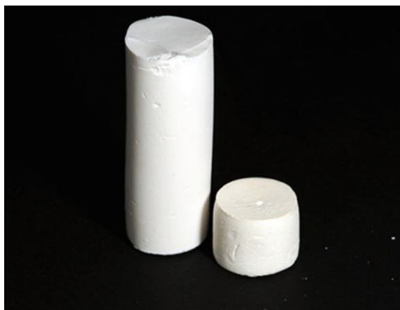
Figure 10.18. Photographs of aerocelluloses prepared from caustic soda solutions of cellulose (cellulose 7% w/w in aqueous NaOH 8% w/w) regenerated in water at 25°C, washed with acetone then dried with supercritical CO 2 . Heights of the samples are, respectively, 3 and 9 cm (courtesy of T. Budtova, MINES ParisTech/CEMEF, Sophia Antipolis, France).
