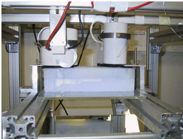
Figure 34.19. The picture shows in the center the Aerogel mold, into which the molten metal enters the wedge-type cavity from the left side (see Figure 34.20, below). A mirror below the shell allows to follow the mold filling and temperature distribution with an infrared camera.
