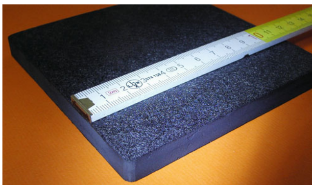
Figure 23.14. Tile of a carbon aerogel for high-temperature thermal insulation with carbon-fiber paper covering layers on both sides to enhance mechanical stability [38].
