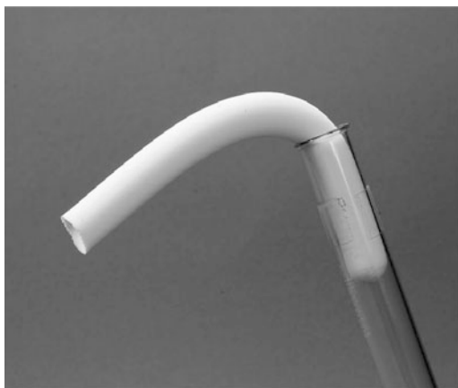
Figure 4.2. MTMS-based flexible silica aerogel.
