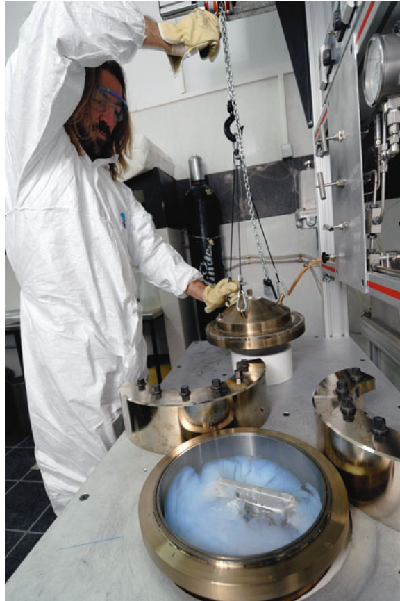
Figure 35.1. The artist is opening the 20 L high-temperature supercritical drying reactor after a 48 h run. The vessel was installed in Greece, September 2005, and all the aer( )sculptures are created since then in it (photograph and copyright: Massimo Pizzocaro 2/2008).
