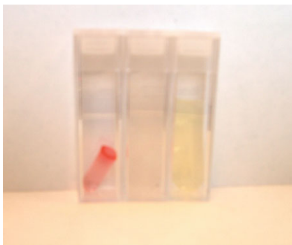
Figure 27.5. Photograph of PtOEP -doped sol-gel materials: xerogel, RSCE aerogel, CSCE aerogel (left to right). Note that the xerogel and CSCE aerogel have the shape of the test tube in which gelation occurred, whereas the cuvette holding the RSCE aerogel sample contains pieces taken from a larger cylindrical monolith. The discoloration of the CSCE aerogel is consistent with results obtained by Leventis for acetone-washed gels [11].
