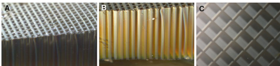
Figure 19.4. Ag patterning of silica aerogels with collimated X-rays. The cell walls have a thickness of 50 \mu\text{m} and the samples are 3-mm thick. From [34]. The images were obtained with a digital camera equipped with a macro objective and they were taken from the same sample.
