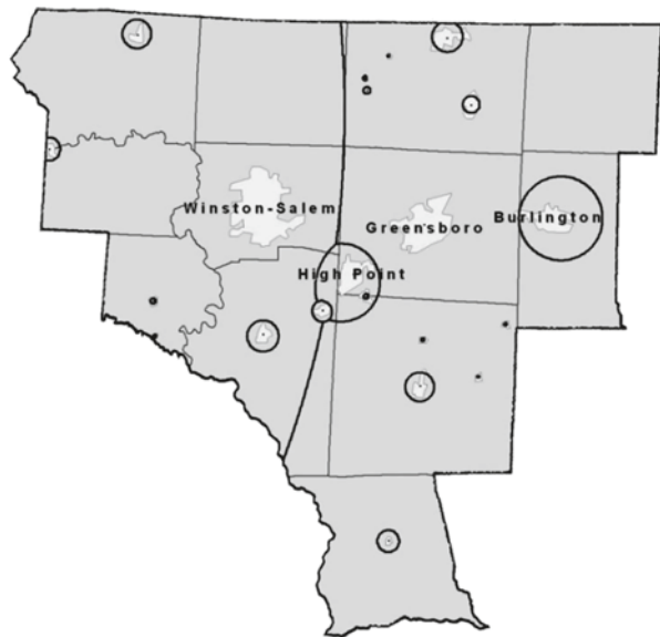
Fig. 19.15 Weighted Voronoi diagram with \ell_2 distances
