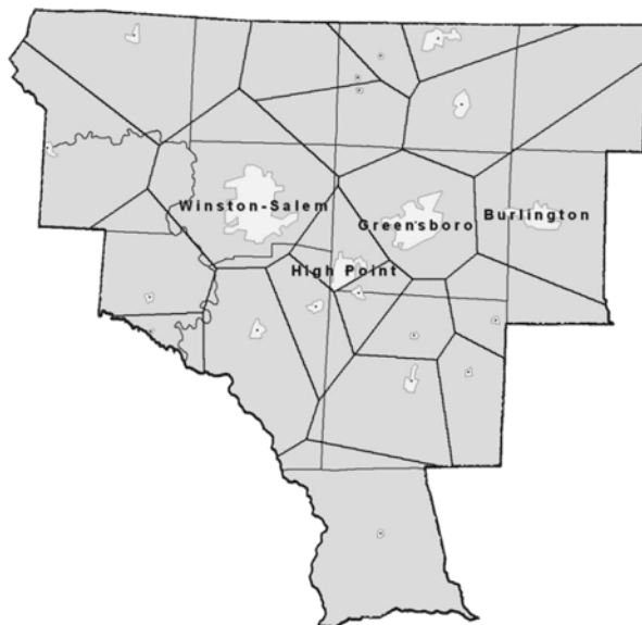
Fig. 19.12 Unweighted Voronoi diagram with \ell_2 distances
