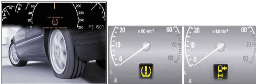
Fig. 4.2 Obligatory in the USA: low tire pressure indication and malfunction indicators
