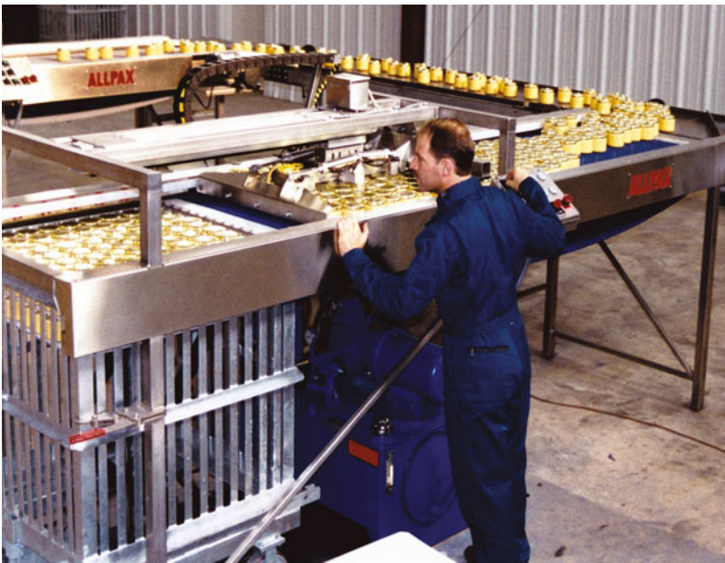
Fig. 11.6 Automated materials handling system for retort basket, rack, or tray loading (Courtesy of Allpax Products, Inc., Covington, LA)
