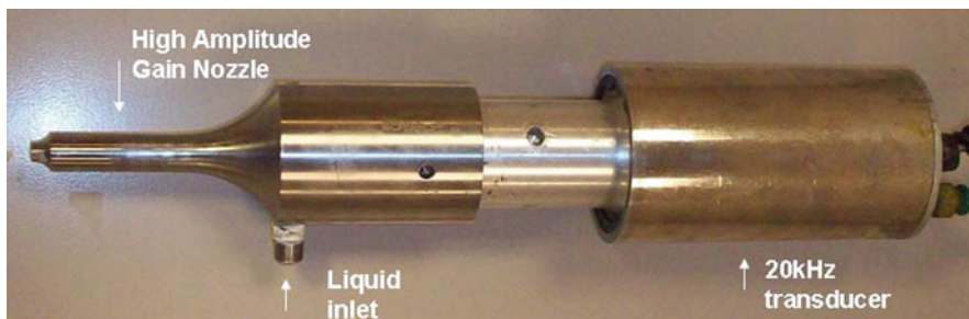
Fig. 20.3 One of the specialty nozzles used for seasoning application
