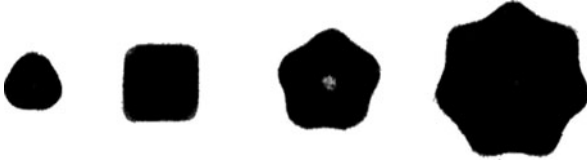
Fig. 2.9 Snapshots of shape unstable bubbles. Reused with permission from Kornfeld and Suvorov (1944, p. 495). Copyright 1944, American Institute of Physics
