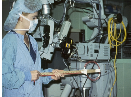
Figure 17.3: Use of a simple wire loop to find the source of magnetic interference (it was the light source for a microscope).
