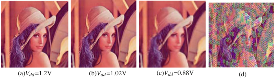
Fig. 8.5 Simulation results at (a) nominal process corner and V_{dd} , (b), (c) SDA DCT at scaled V_{dd} , (d) conventional design under scaled V_{dd} or variations
