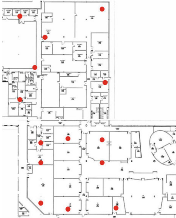
Fig. 7.5 Office environment test bed with anchors
