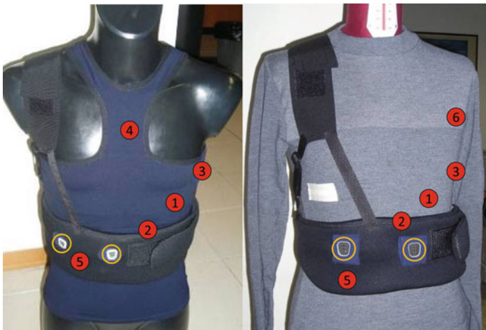
1-Textile electrodes (heart rate sensor); 2-Piezoelectric cable (breathing rate sensor); 3-Body temperature sensor (under the left armpit); 4-blood oxygen saturation sensor (on the CP version only); 5-Vital signs board (IG electronics); 6-dehydration sensor.
