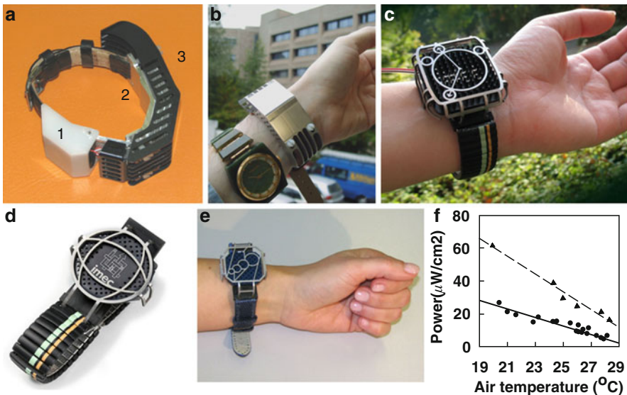
Fig. 2.8 (a) The first wrist TEG: (1) is the electronics module, (2) is a hot plate, and (3) is a radiator. (b) A similar TEG worn next to a watch. (c) A TEG with a pin-feathered radiator. (d) A waterproof TEG for outdoor use. (e) A TEG in the wireless sensor for measuring the power generated by people in real life. (f) The power produced by the device shown in (c) in the office on a sitting ( circles ) and walking ( triangles ) person
