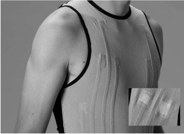
Fig. 7.1 Knitted intarsia electrodes and textile connections, particularly on the skin side on the right
