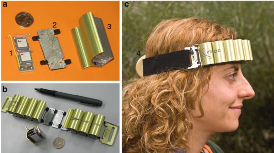
Fig. 2.10 Wireless electrocardiography system powered by the body heat: (a) and (b) show the TEG components in the assembling stage, and (c) is a completed device. (1) is a thermopile module, (2) is a hot plate, (3) is a radiator and (4) is the electronics module
