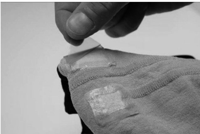
Fig. 7.2 Hydrogel membrane coupled with textile electrode
