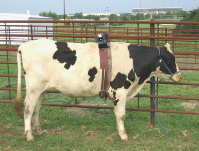
Fig. 3.4 Wearable, wireless cattle health monitoring system that acquires core body temperature, heart rate, three acceleration axes, ambient temperature, ambient humidity, and global position (Nagl 2004; Smith et al. 2006; Warren et al. 2008a, 2008b)
