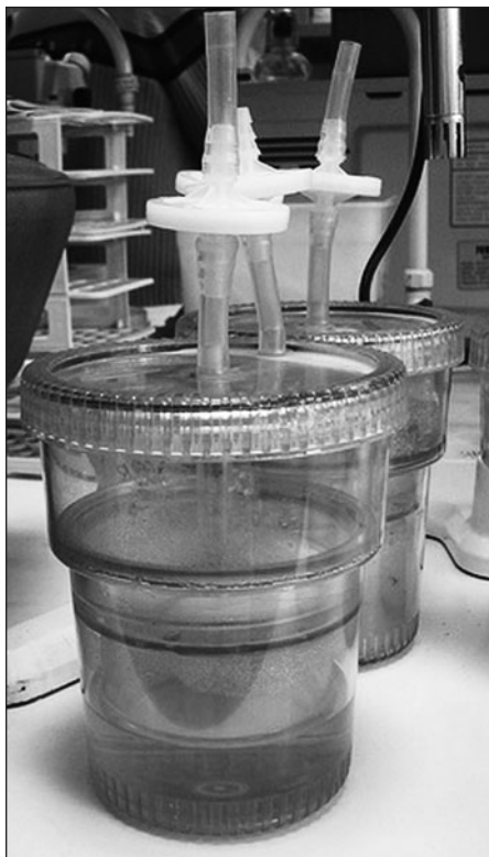
Figure 4. Temporary immersion system (RITA ® , Vitropic, Saint-Mathieu-de-Trévières, France) for cultivating hairy root cultures.
