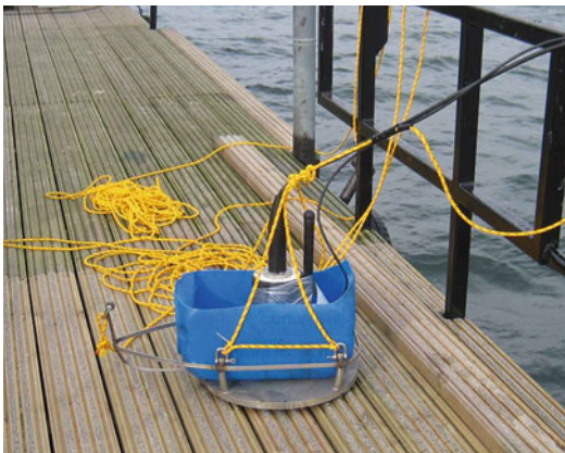
Figs. 3 and 4 Tests conducted at the National Physical Laboratory's (NPL) Wraybury calibration facility used a triple geophone set. The additional plastic “hull” minimizes the risk of it sinking too far into the soft Wraybury sediment
