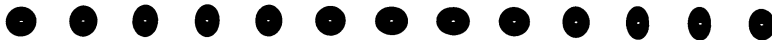
Fig. 26.1 Stream of monodisperse propanol-2 droplets with highly controlled size, as produced with a droplet stream generator of the presently discussed kind. The oscillations are caused by the deformations upon pinch-off from the jet
