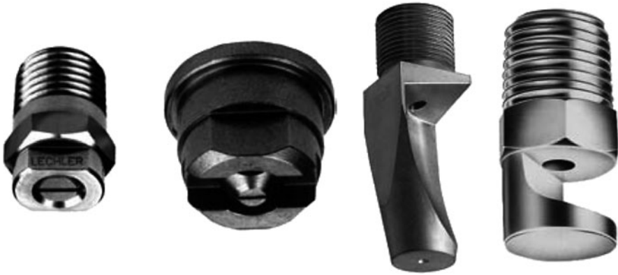
Fig. 24.27 Examples of flat fan nozzles. The two on the left use axial flow, while the two on the right use tangential flow (Courtesy of Lechler, Inc.)
