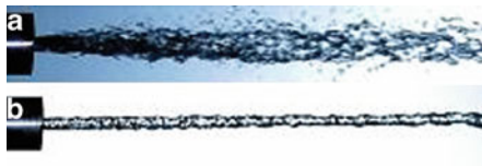
Fig. 10.9 (a) The temperature is below the boiling point and the jet breaks due to instability of a circular jet. (b) The temperature is 10°C degrees above the boiling point. The jet is not intact anymore
