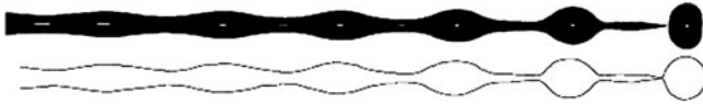
Fig. 18.11 (Above) Axisymmetric breakup of a weakly electrified jet in the experiments compared to (below) the results of the corresponding numerical simulation using a 1D model [76, 77] (Courtesy of Elsevier)
