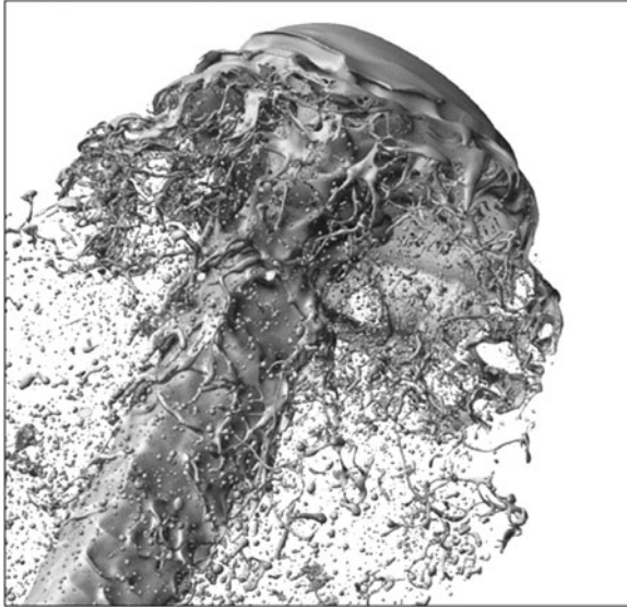
Fig. 17.9 Direct numerical simulation of a liquid jet at high speed injected into still air [30] (Courtesy of Elsevier)
