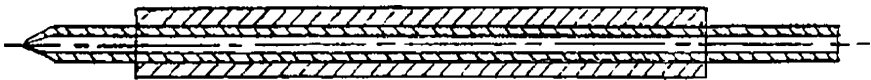
Fig. 25.6 Drawing of a piezoceramic tube with imbedded capillary (Reprinted from [37]. With permission. Copyright 2001 Wiley)
