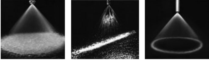
Fig. 24.5 Three common spray shapes: full cone ( left ), flat fan ( center ), hollow cone ( right ) (Courtesy of Lechler, Inc.)
