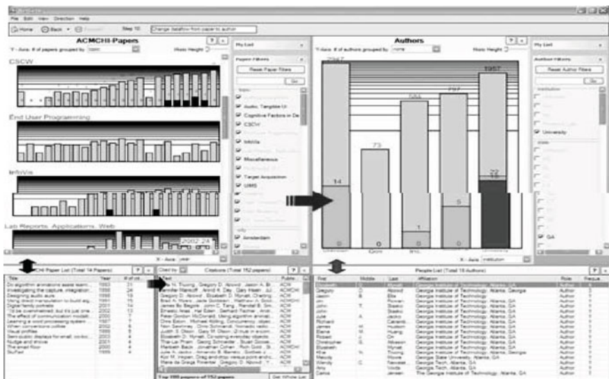
Fig. 28.8 A screenshot of NetLens, an interactive system to explore networks using simple bar charts. Users filter different attributes of the network by clicking on corresponding bars. NetLens provide the textual result on the lower windows
