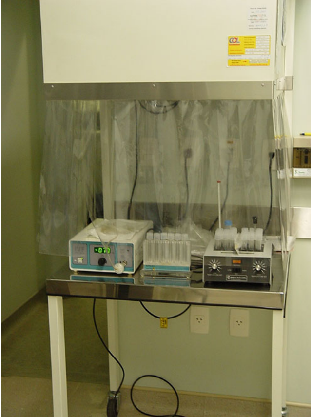
Fig. 9.17 Portable minihood containing a high-efficiency particulate air (HEPA) filter
