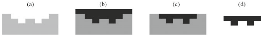
Fig. 2.36 [174] (a) micromold, (b) SiC deposited micromold, (c) micromold with SiC after removing excess SiC, and (d) released SiC microstructure (©Elsevier 1999), reprinted with permission.
