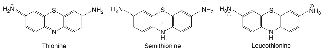
Photogalvanic Cells, Principles and Perspectives, Fig. 5 The three structures of the thionine dye within the iron-thionine PG system
