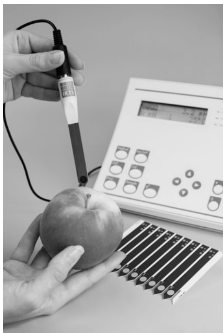
pH Electrodes - Industrial, Medical, and Other Applications, Fig. 4 Thick film pH glass electrode
