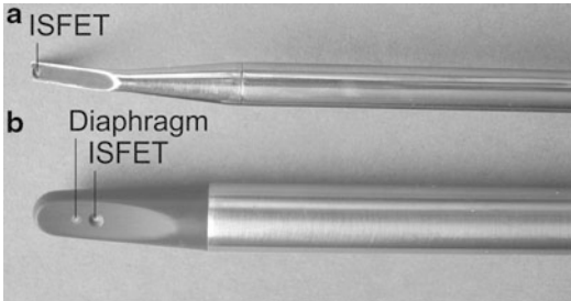
pH Electrodes - Industrial, Medical, and Other Applications, Fig. 6 ISFET pH probes for measurements in stomatology (a) and gynecology (b)
