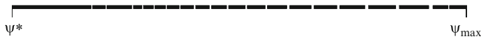
Fig. 2.11 Chaotic repeller associated with shimmying motion on the angle interval (\psi^*, \psi_{\max}) = (6, 9) degrees
