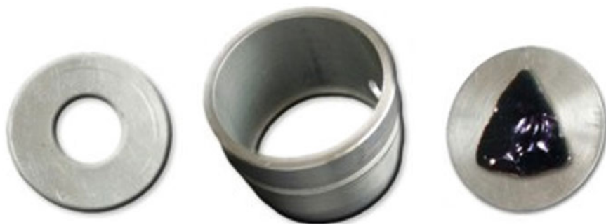
Fig. 5.2 The sample container of the PW 1480 XRF and an integral obsidian fragment positioned for non-destructive analysis
