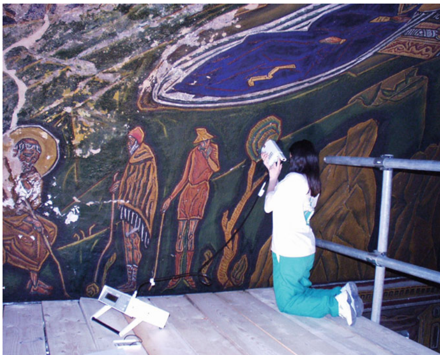
Fig. 6.1 Spectrace 9000 TN PXRF measuring mural paintings of modern artist Spyros Papaloukas from the Amfissa Cathedral, near Delphi, Greece
