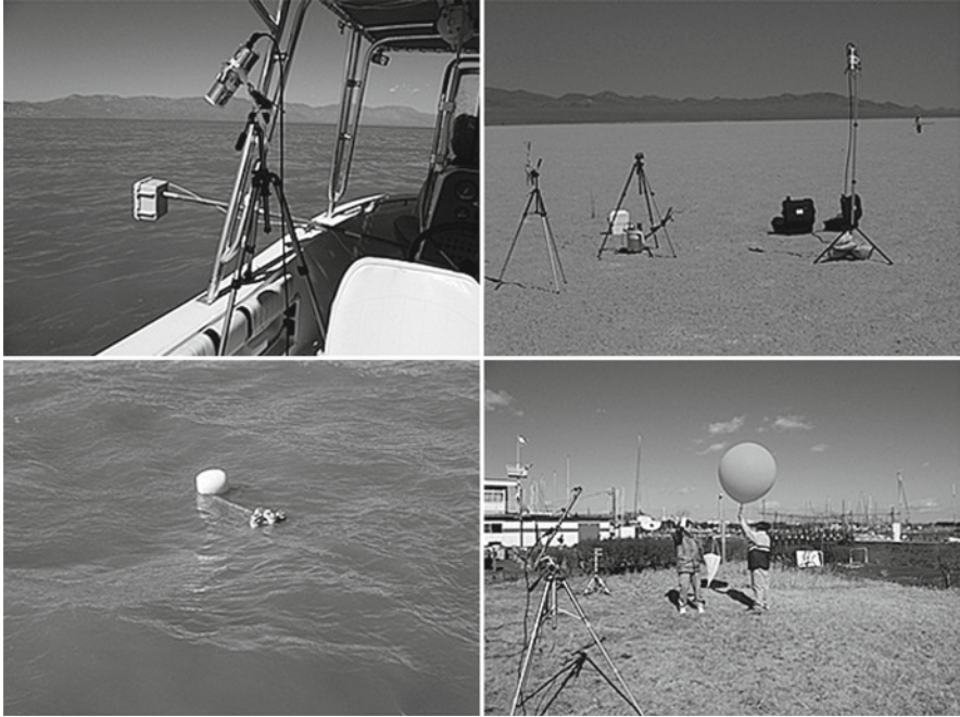
Fig. 6.5 Photos from VC experiments. Upper: multi- and single-band radiometer measurements at Salton Sea, CA ( left ), and Alkali Lake, NV ( right ). Lower: thermistor measurement ( left ) and radiosonde measurement ( right ) at Lake Kasumigaura, Japan
