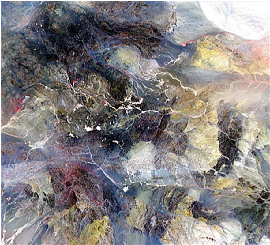
Fig. 14.14 View of southern Gobi project area using an ASTER color-infrared composite (Bands 3, 2, and 1 in RGB). Red reflects vegetation, yellow/green represent red-colored rocks and soils, black is dark-colored exposures, and white indicates evaporitic salts or bright sediments in drainage. The image is orthorectified to UTM/WGS-84 map base and measures approximately 54 km in width
