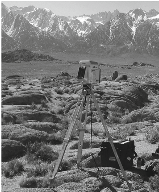
Fig. 20.4 Ground-based 3D laser scanner (Trimble GS200) used in this study. To achieve the high-resolution mapping required for this study (i.e., <5 mm postings), each surface required multiple (~3–5) measurements of the scene from different view angles, to overcome the problem of areas hidden behind roughness elements at the grazing view angles of a ground-based system
