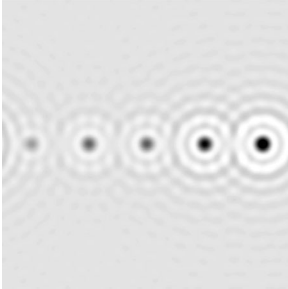
Fig. 5.12 The coherent bright field phase contrast image of five isolated single atoms and an incident electron beam energy of 200 keV. The electron optical parameters are spherical aberration C_s = 1.3 mm, defocus \Delta f = 700 Å and an objective aperture of 10.37 mrad (Scherzer conditions). This was calculated with a sampled image of 512 \times 512 pixels. Atomic number Z = 6(\text{C}), 14(\text{Si}), 29(\text{Cu}), 79(\text{Au}), 92(\text{U}) (left to right). The image ranges from 0.72 ( black ) to 1.03 ( white )
