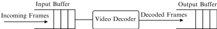
Fig. 7.25 I/O buffering for video decoder: since decoding time varies from frame to frame, the input buffer is needed to hold the frames streaming in. All the decoded frames are buffered into the output buffer until the GOP is completely rendered, and only then the decoded frames of the entire GOP are streamed out
