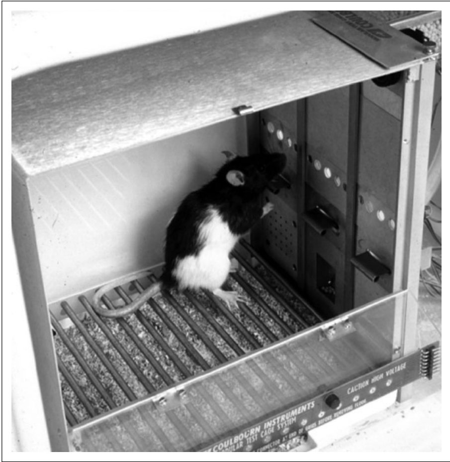
Figure 1. Standard operant chamber containing response levers, feeder (behind panel) and stimulus lights.
