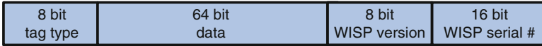
Fig. 2 Structure of the 96-bit ID used to transmit sensor data within the ID
