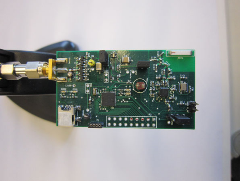
Fig. 7 WARP sensor node consisting of a rectifier, power management circuitry, sensors, and 2.45 GHz transceiver with ceramic chip antenna (power-harvesting antenna not shown)
