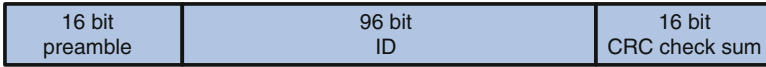
Fig. 1 Structure of a 96-bit ID tag reply according to the EPC Class-1 Generation-2 UHF RFID protocol
