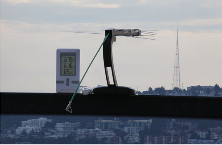
Fig. 2 Demonstration of a temperature and humidity meter (including LCD display) that is exclusively powered from ambient RF signals transmitted by the TV tower seen in the background, at a distance of 4.1 km
