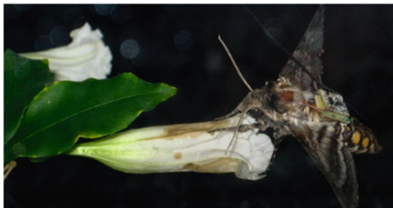
Fig. 20 Photograph showing an untethered moth with the RFID measurement sensor
