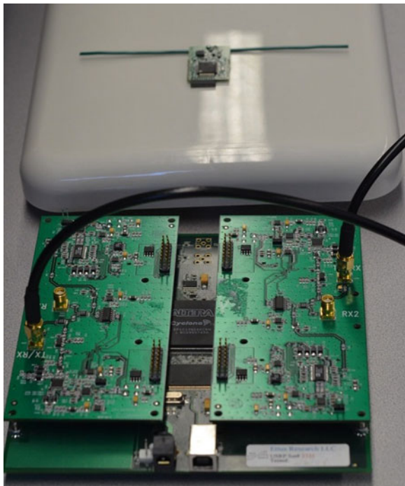
Fig. 5 Hardware used to implement BAT. The relay ( foreground ) is a USRP with RFX900 daughterboards driven by GNU Radio. The UMass Moo ( background ) is a CRFID tag derived from the DL WISP 4.1 [23]
