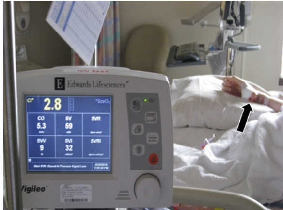
Fig. 31.3 The Vigileo Monitor (Edwards Lifesciences LLC, Irvine, California) extracts data from a radial artery catheter (arrow) to provide reliable estimates of stroke volume (SV), cardiac output (CO) and stroke volume variability (SVV)
