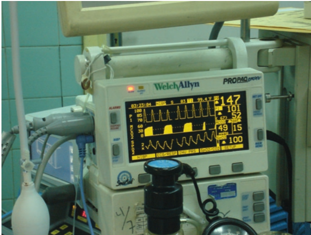
Fig. 31.1 Ubiquitous portable monitoring unit used in deployed Army surgical units. Continuous electrocardiographic tracings, pulse oximetry, temperature, and respiratory rate are standardly displayed. This particular monitor also reveals end-tidal CO 2 monitoring in an intubated patient
