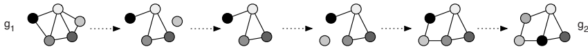
Figure 7.6. A possible edit path between graph g_1 and graph g_2 (node labels are represented by different shades of gray).
