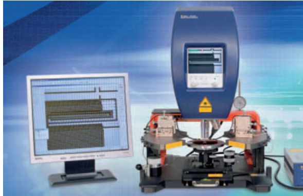
Fig. 6.13 Polytec MSA-500, on a Cascade Microprobe Test Station. Reprinted with permission. Courtesy Polytec GmbH
