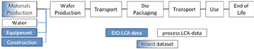
Fig. 7.1 Life-cycle stages with data source types [1]
