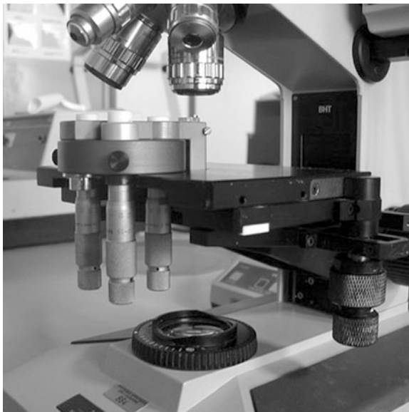
Fig. 4.43 Microscope with modified stage for placing the tripod tool
