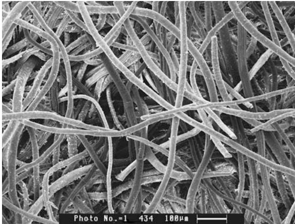
Fig. 2.14 Structure of an unweaved cloth
