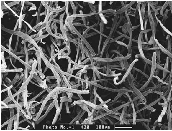
Fig. 2.15 Structure of a flocked cloth
