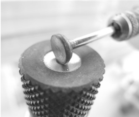
Fig. 2.18 The grinding wheel ( vertical ) on the rotating thin slice ( horizontal )
