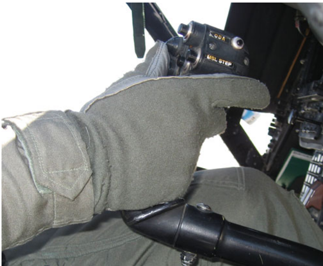
Fig. 6.39 Side photo showing typical hand position relative to cyclic rest. One can see the energy transfer of the fifth MC as it impacts the rest during sudden deceleration and downward force from a crash
