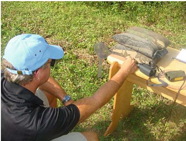
Fig. 5.65 In this figure, I am determining the angle of the sniper bench with a clinometer. We also measured the zeroed-out barrel of the weapon just prior to shooting downrange at the target (Photo by Dr. Mike Frew)
