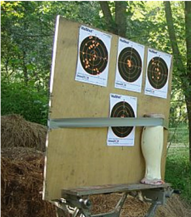
Fig. 5.67 The anatomic ballistic model was fastened to a stable bench as the target. Various known sniping angles were accomplished (Photo by Dr. Les Folio)
