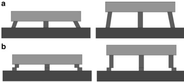
Fig. 5.13 (a) Using high bumps can reduce the strain of solder joints, but (b) it has much less influence on the strain of ACA joints
