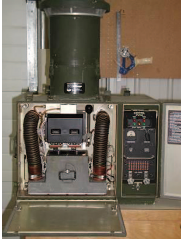
Fig. 2.2 XM2 was a liquid based sampler that sequentially impinged aerosol particulates into two liquid containing plastic containers. The system could take a series of two samples after being triggered by the XM19
