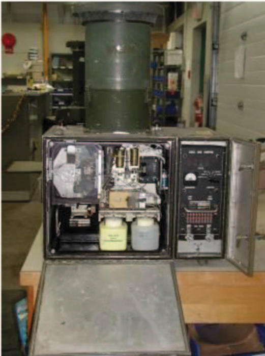
Fig. 2.1 XM19 biological detector showing virtual impactor, tape cassette, liquid chemistry, electronic sensor and analogue electronic panel
