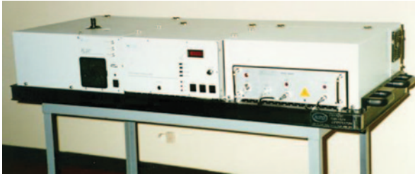
Fig. 2.7 The prototype Fluorescence Aerodynamic Particle Sizer, also called version 1 (FLAPS1). In the center is seen the APS electronics with its familiar face plate. On the right is the large power supply used to drive a HeCd laser which was located at the back of the unit, essentially occupying the length of the system. Additional optical elements were located on the left side to focus and direct the UV beam to the APS aerosol box. The aerosol intake can be seen protruding from the left top panel . A Newport optical bench provided stability to the optical and electronic elements. This was essential for long distance transport to field trial locations
