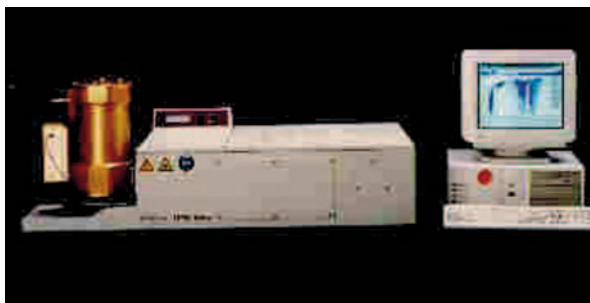
Fig. 11.6 Bruker IFS-66 spectrometer with an Hg-lamp source and He cooled Si-bolometer (1.7°K). Three vacuum systems are not shown
