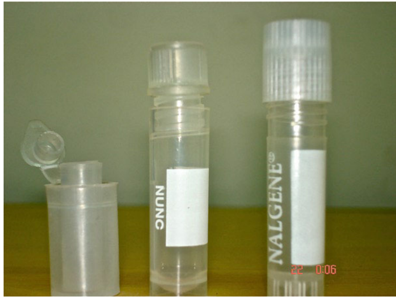
Fig. 31.1 Commercially available vials for semen packaging. Cryotubes may have internal or external threads. Few of these may have an external reservoir for liquid nitrogen for better temperature maintenance
