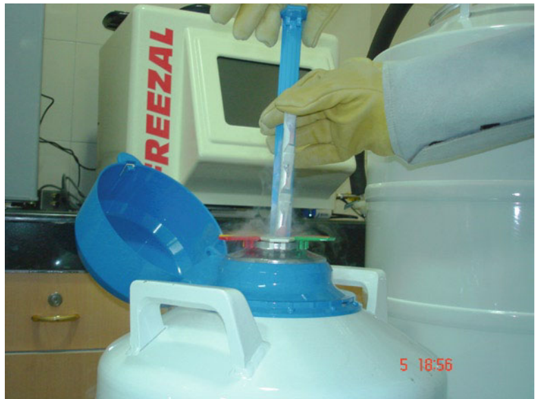
Fig. 31.3 Semen containing vials being loaded on the aluminum canes before being dipped in LN 2 in the cryocontainers
