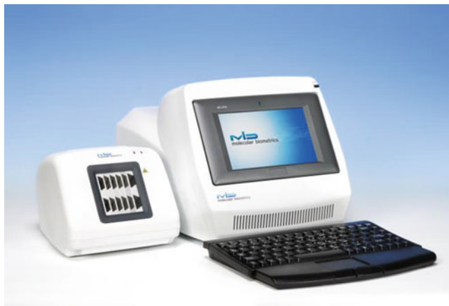
Fig. 44.2 The ViaMetrics TM instrumentation. The temperature stabilizer is on the left , and instrument is on the right (courtesy of Molecular Biometrics, ©2010 Molecular Biometrics, Inc.)
