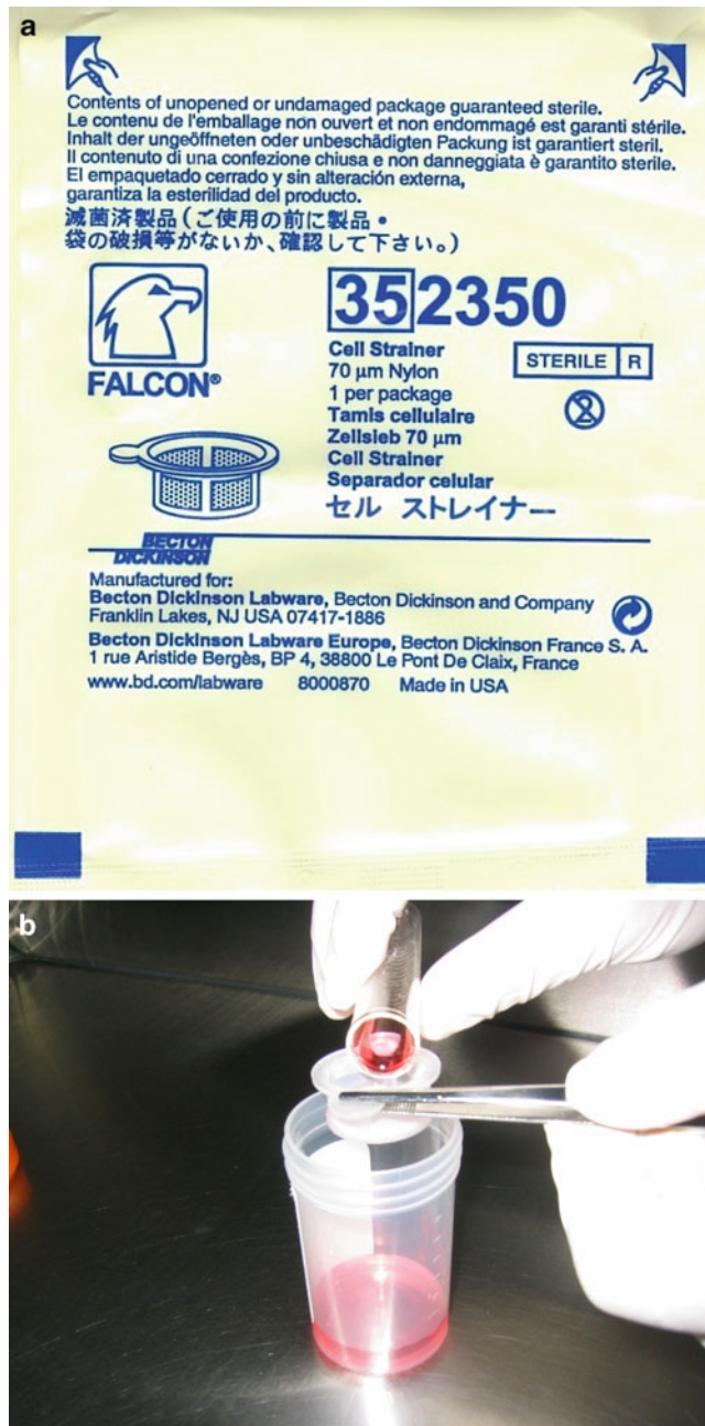
Fig. 18.1 (a) Labeling on Cell Strainer (Falcon, Becton Dickinson and Company, USA); (b) follicular aspirates are filtered with a Cell Strainer
