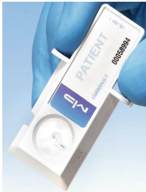
Fig. 44.3 A sample cell that is used to scan the embryo culture media and control media. There are two small injection ports on the side
