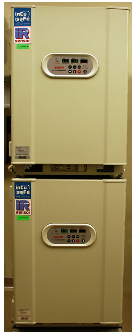
Fig. 9.2 A 170 L infrared CO 2 sensor, conventional air-jacketed incubator. Faster CO 2 recovery can be expected with a large infrared sensor-equipped incubator than with a smaller incubator with a thermoconductivity CO 2 sensor
