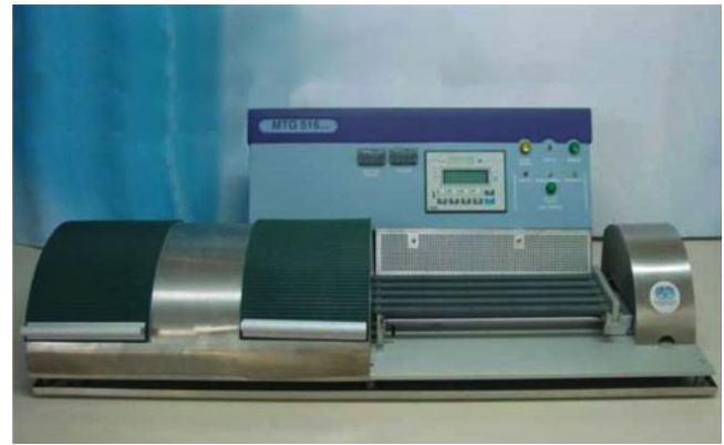
Fig. 60.2 Multi gradient thermal device in which large volume test tubes with samples are advanced at a constant velocity through a predefined temperature gradient to achieve optimal heat transfer and extracellular ice crystallization
