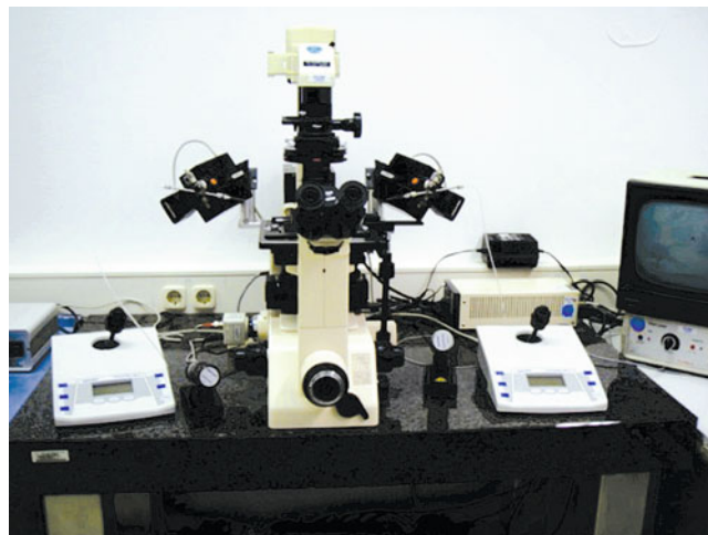
Fig. 37.1 The Eppendorf micromanipulator is composed of three main components: motor module unit, control board, and main power supply
