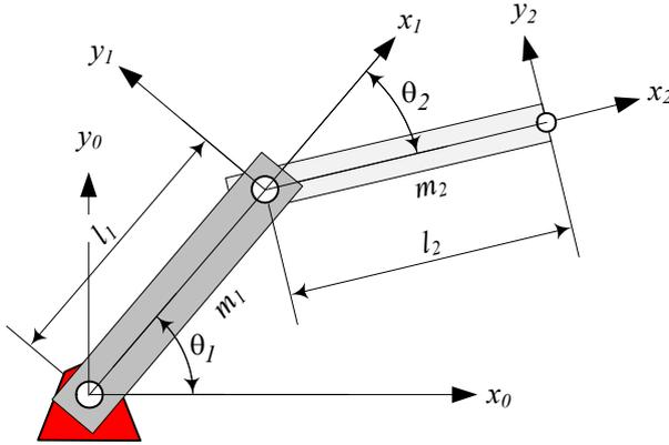
FIGURE 12.20. A 2R planar manipulator with massive links.
