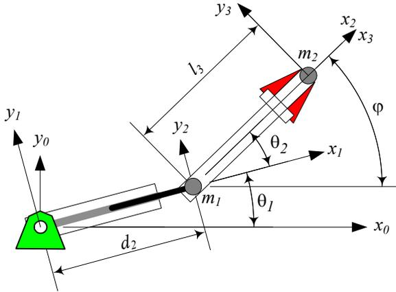
FIGURE 12.27. A *RPR* planar redundant manipulator.
