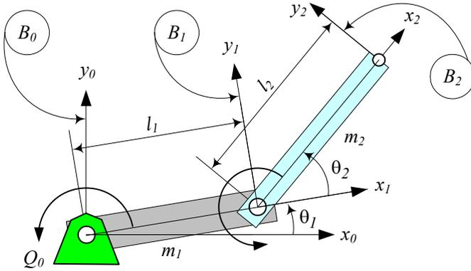
FIGURE 12.14. A 2R planar manipulator with massive links.
