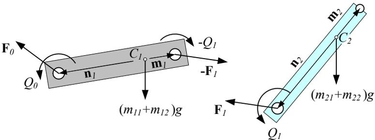
FIGURE 12.9. Determination of the vectors  $\mathbf{m}$  and  $\mathbf{n}$  for new positions of mass center  $C_i$ .
