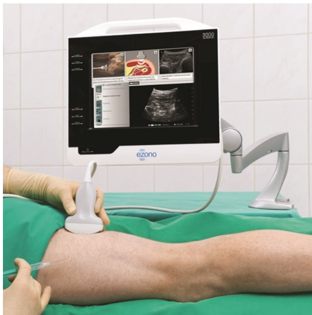
Figure 4.9. Real-time and image interpretation support system (eZONO). The eZONO device allows the operator to use a bank of stored preset images and video, and anatomical cross sections which can be used during the procedure of choice to provide a real time on-hand high quality reference and image interpretation support. Used with permission from eZONO.
