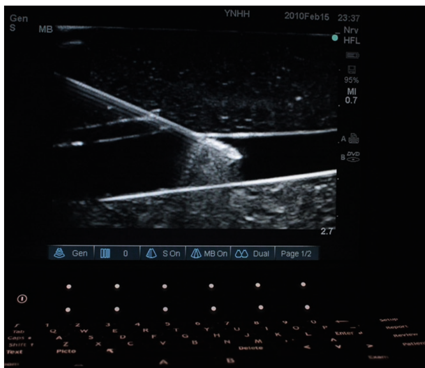
Figure 4.35. Needle enhancement. Needle enhancement within the vessel wall occurs because of an increased difference in acoustic impedance between needle and vessel fluid. The needle shaft at the site of entry into the vessel wall does not enhance as brightly as the tip within the vessel wall.
