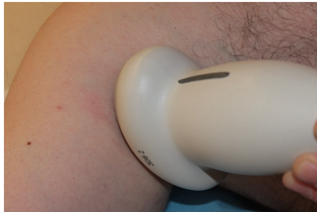
Figure 4.24. 3D needle ultrasound and needle visibility. This is a 3D ultrasound probe. Currently 3D ultrasound probes are larger than their 2D counterparts. However, newer, smaller 3D ultrasound probes are in development.
