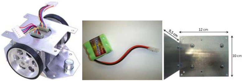
Fig. 2 Mechanical block: it is composed out of two engines, two wheels, a battery pack and a metal platform to host the mobile phone
