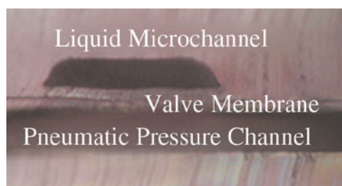
Fig. 5.15 Cross-sectional view of the fabricated PDMS microvalve
